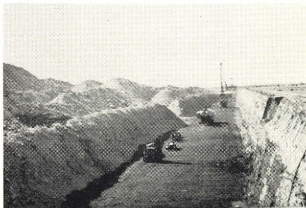
Here is strip pit coal mining in actual operation. Many of the lakes of southeast Kansas have been formed from pits such as these. They gradually fill with water through seepage and surface runoff and trees and other vegetation grow on the high banks.
